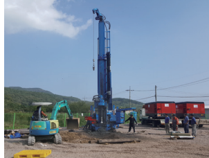
Deep drilling (1km) for borehole sensors
