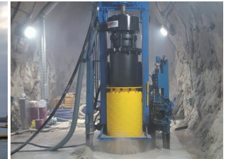
Large-diameter (φ900mm) drilling
