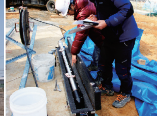
Installation of deep borehole seismic sensors
